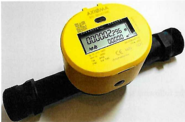
Fig. 3. Water meter QALCOSONIC W1, Q_3 = 6,3/10 \text{ m}^3 , with threaded end connection G 1¼ or G 1½
