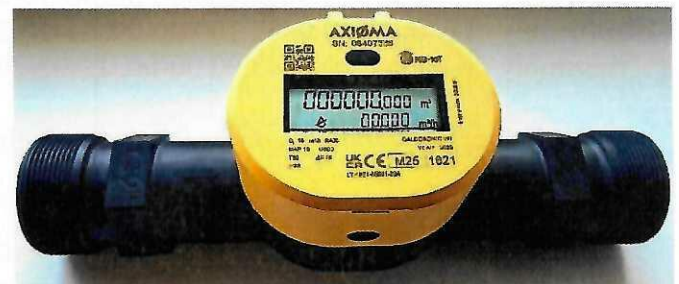
Fig. 3. Water meter QALCOSONIC W1, Q_3 = 10/16/25 \text{ m}^3 , with threaded end connection G2
